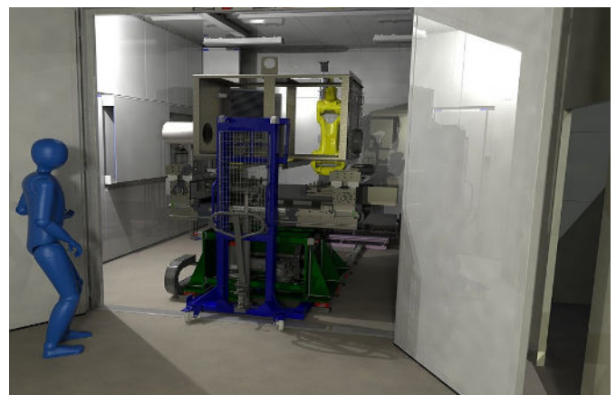
View of the enclosure where all of the internal surfaces (including the doors) have Laser Jailer active guarding fitted.
