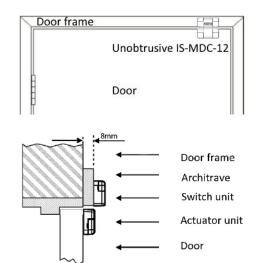
High tolerance to offset alignment. Up to 8mm difference between the door and the door frame/architrave can be tolerated as shown here
