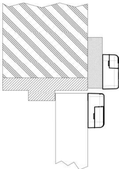
The part with the Lasermet badge and the cable attached (known as the switch) is normally affixed to the door frame, and the other part (known as the actuator) is attached to the door. The fixing hole positions are shown above and the usual mounting arrangement on a door on the left.
