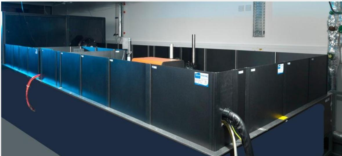
***Being modular, Optoblok can be used on all sizes of optical tables***
