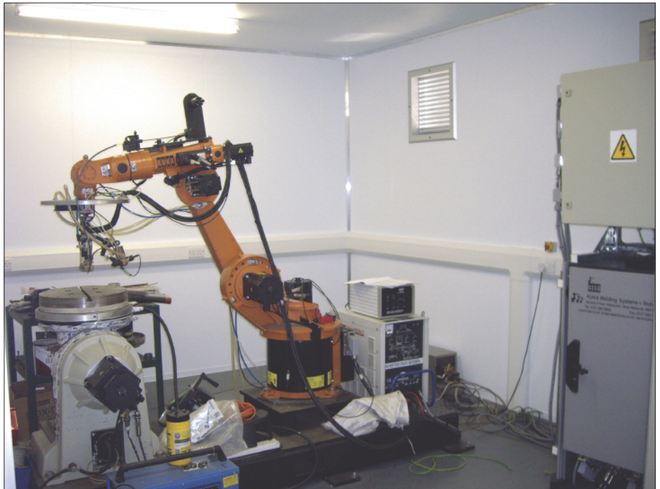
Inside view showing robot mounted laser and laser-safe air vents
